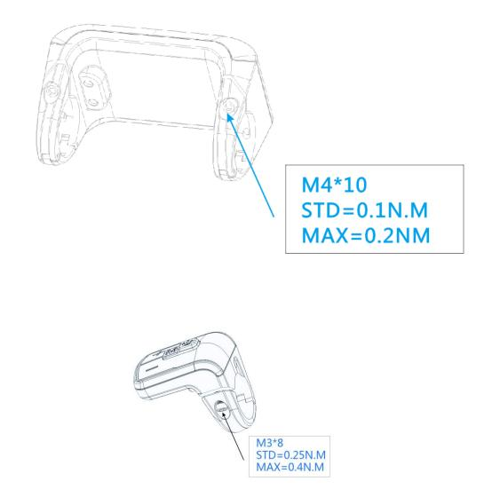
Clamps suit for 3 size of handlebar, 31.8mm, 25.4mm, 22.2mm, there are transfer rings for
