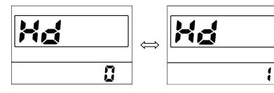
**8.10 Magnetic pole numbers of speed sensor (HAL):** Press UP/DOWN can change the parameter from 1 to 15(common value is 1 or 6).
