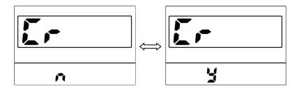
8.2 System (S7): Press Up / Down button to switch between Metric / Imperial.
