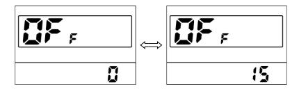
**8.5 Wheel (dH):** Press UP/DOWN can change the wheel setting, optional wheel diameter is 16/18/20/22/24/26/27/28/700C/29 inch.
