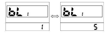
**8.4 Auto off (Off) :** Press UP/DOWN button to change the auto power off time, from 0 to 15, the number represent time (minutes) to shutdown, default value is 5 minutes.
